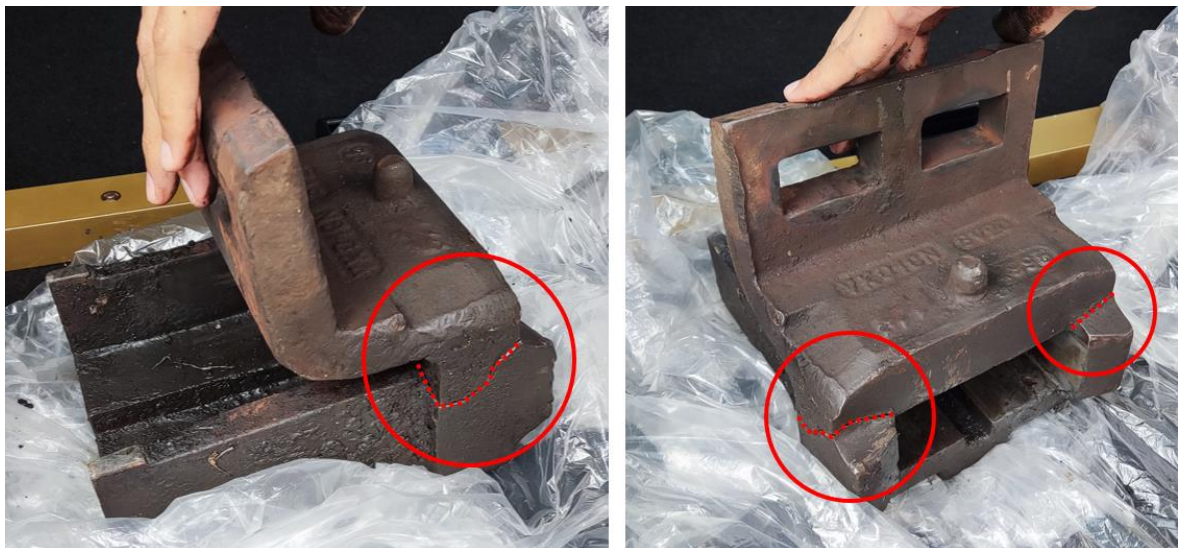
Gambar 6. Lockbox wesel 1 patah
