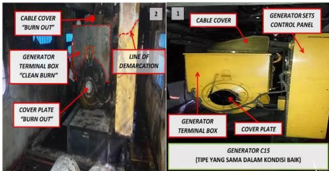
Gambar 29. Clean Burn & Line of Demarcation
