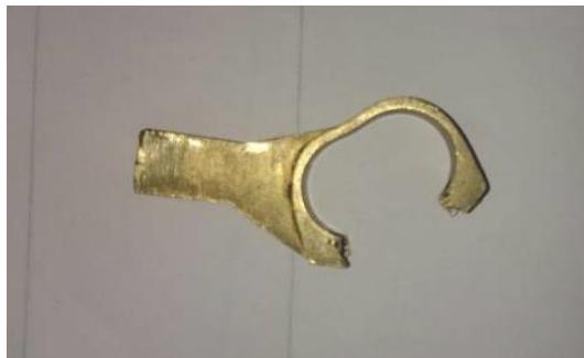
Gambar 4. Sentil No.19F mistar 25 patah
