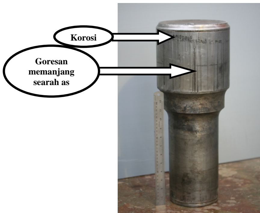
Gambar 6. Patahan As Sisi Keping Roda
