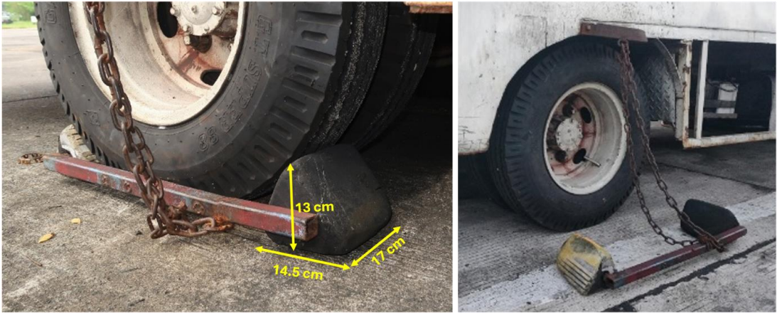
Figure 7: The dimension wheel chock of the LST (left figure) and the chained position of the wheel chock (right figure)
