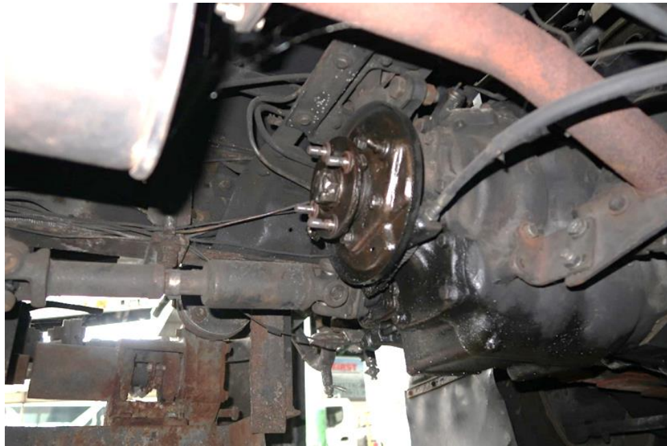
Figure 11: The parking brake drum without internal components
