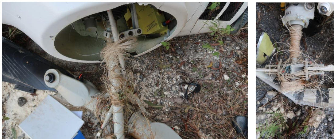
Figure 9: The kite string on the main rotor and tail rotor mast
