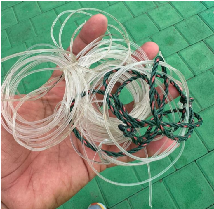
Figure 16: The kite string and plastic rope that were removed from the main rotor and tail rotor masts
