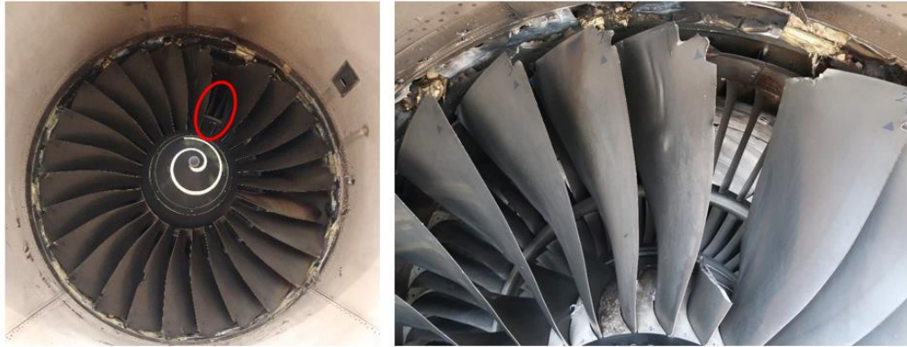
Figure 1: The fan blade release and heavy rubbing around the fan case.
