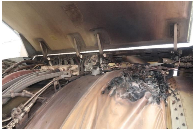
Figure 2: The damage to the Kevlar layer
