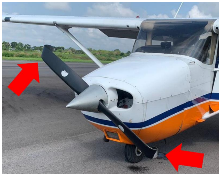
Figure 3: Damaged propeller blades
