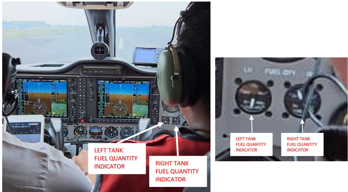
Figure 1: The flight deck view during take-off roll at Pondok Cabe and the zoom in of the fuel quantity indicators
