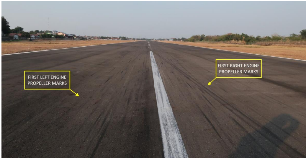
Figure 7: The propeller marks found on the runway
