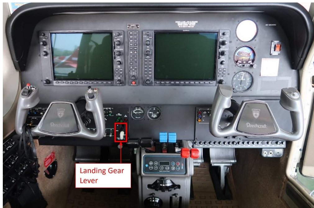
Figure 2: The landing gear lever position
