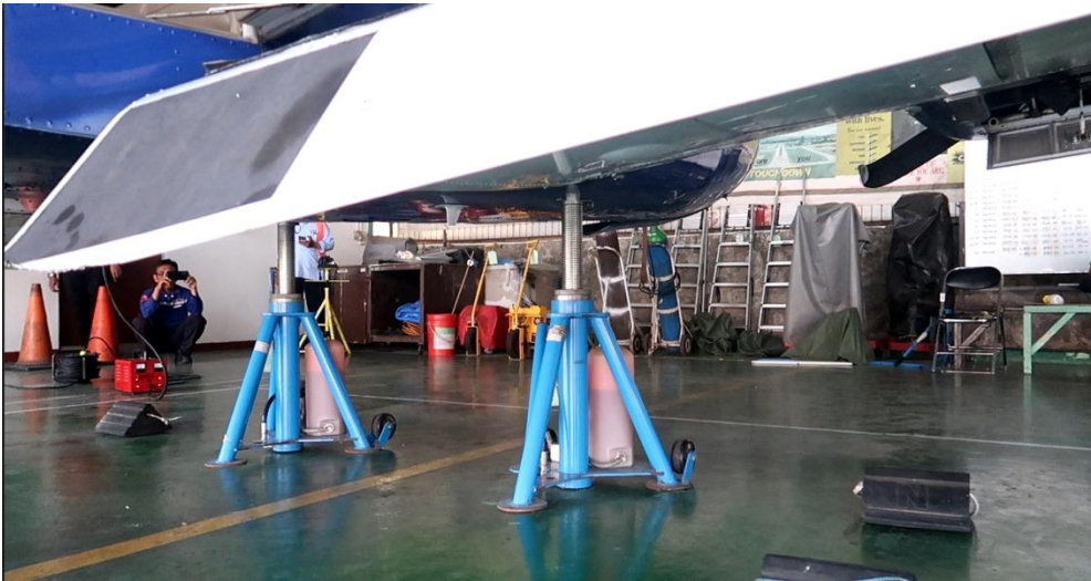
Figure 13: The landing gears were in the up position while the flap was extended
