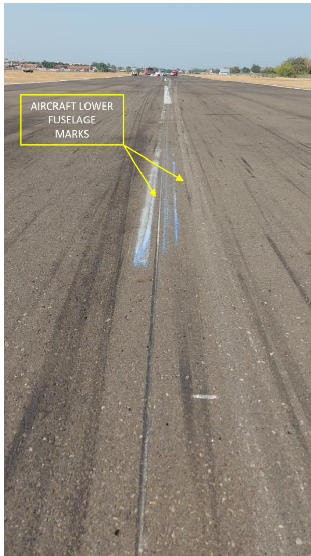
Figure 8: The aircraft lower fuselage marks found on the runway
