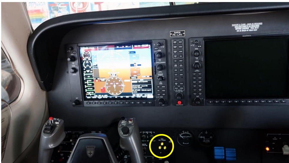
Figure 11: The yellow circle showed the three green lights were illuminated
