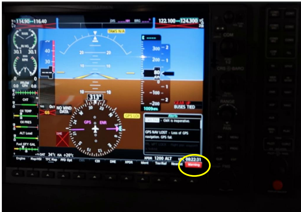
Figure 15: The yellow circle indicates the red warning in the PFD
