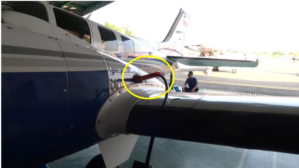
Figure 10: The yellow circle showed the external power source was attached to the aircraft
