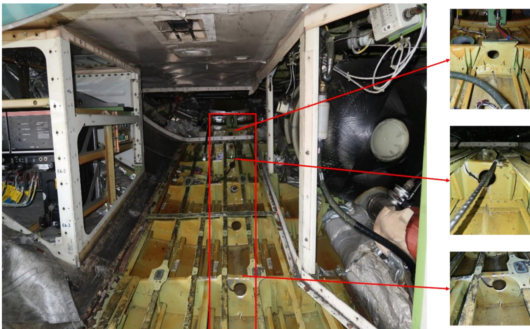
Figure 2. Internal damage on lower surface of the aft fuselage
