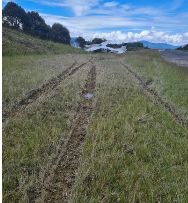
Figure 8: The aircraft tire marks outside the runway
