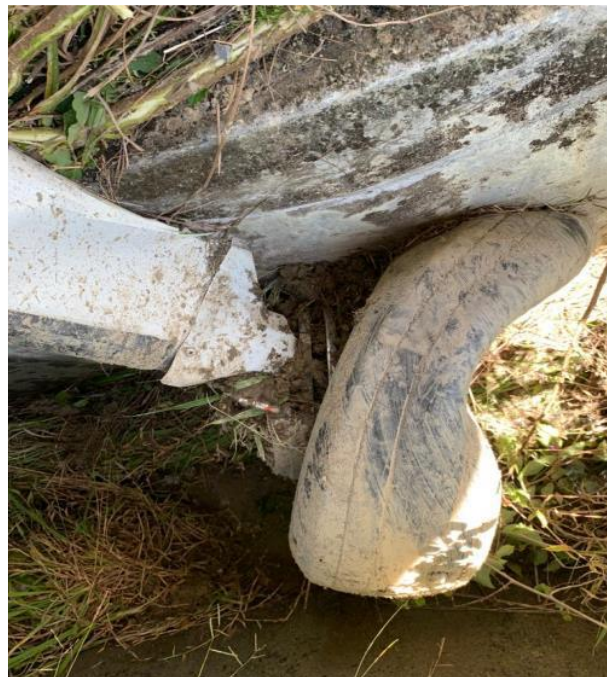
Figure 2: Left main landing gear tire burst and fairing damage
