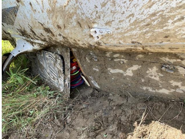
Figure 3: Cargo pod C and D damage
