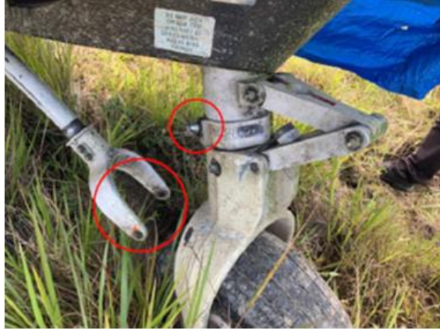
Figure 1: Bolt AN6-52A shear cutoff and fork draglink spring bearing come out
