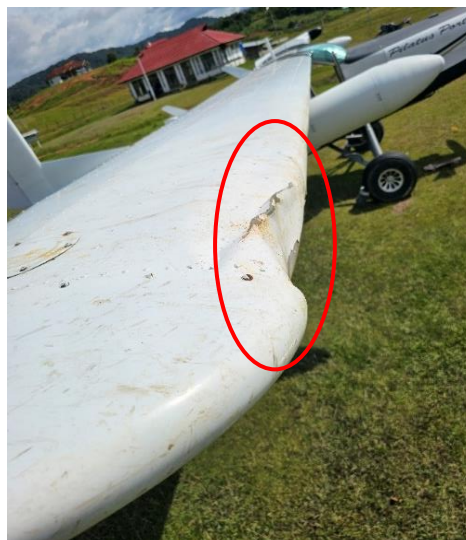
Figure 3: Dent on the leading edge of right wing (red-highlighted). View from right hand side of the aircraft (looking inboard).
