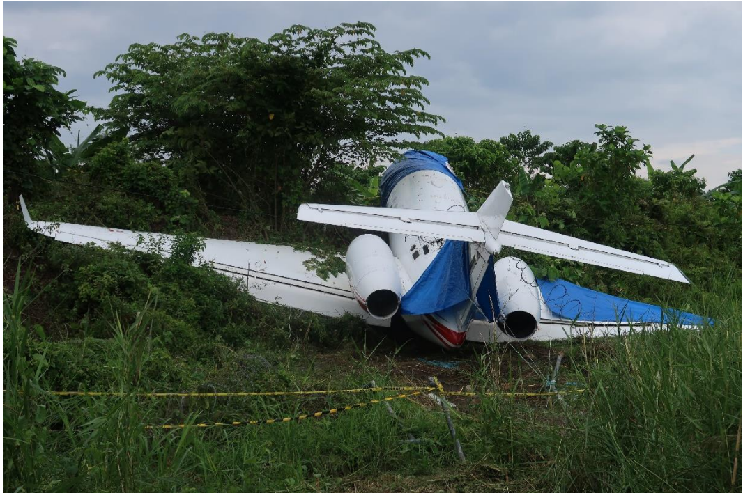
Figure 7: The engine thrust reversers dan air brake position
