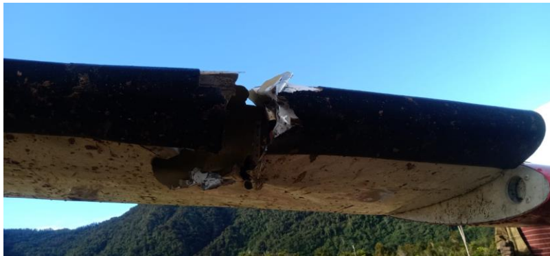
Figure 5. Damaged leading edge of left horizontal stabilizers
