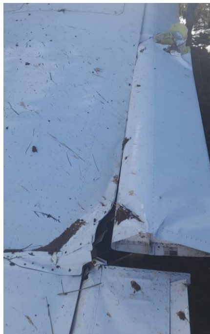
Figure 3. Damaged left wing (view looking inboard)
