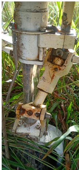
Figure 6. Broken nose landing gear torque link
