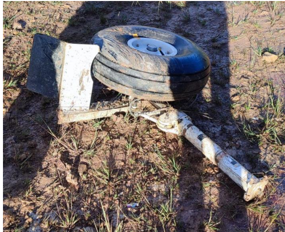
Figure 9. The detached left main landing gear
