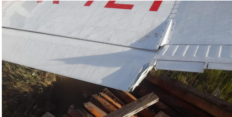
Figure 4. Damaged right wing (view looking forward)
