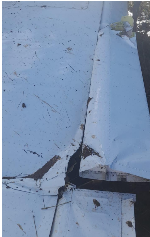
Figure 4: Damaged left wing (view looking inboard)
