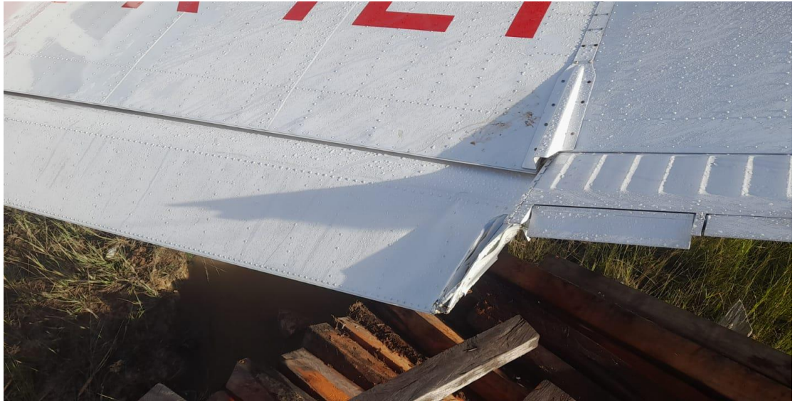
Figure 5: Damaged right wing (view looking forward)
