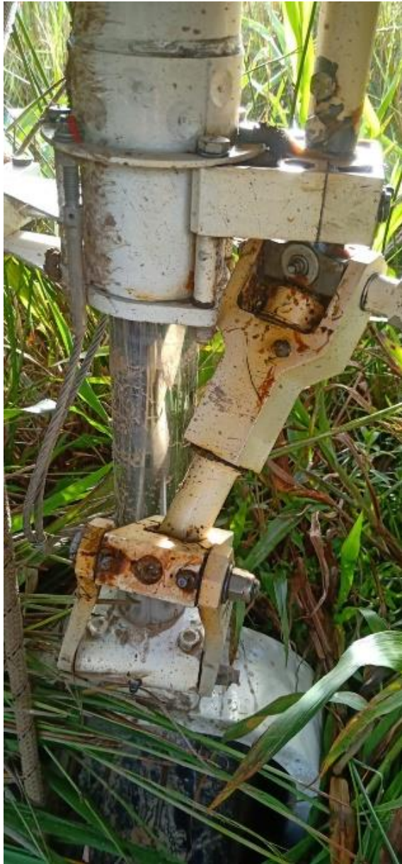
Figure 7: Broken nose landing gear torque link
