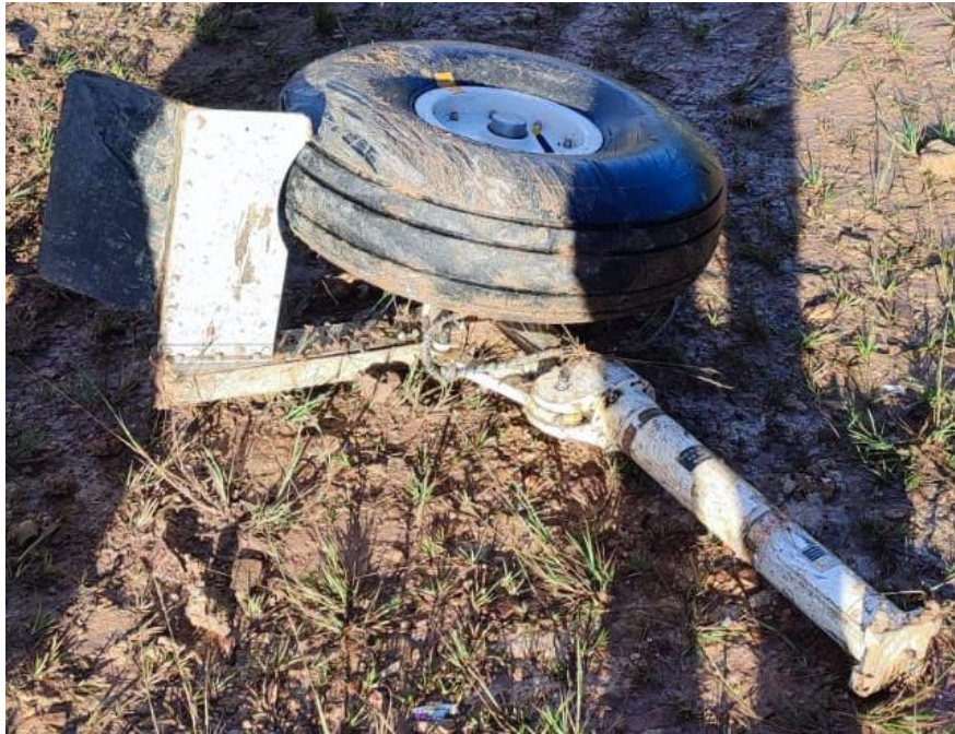
Figure 8: The detached left main landing gear
