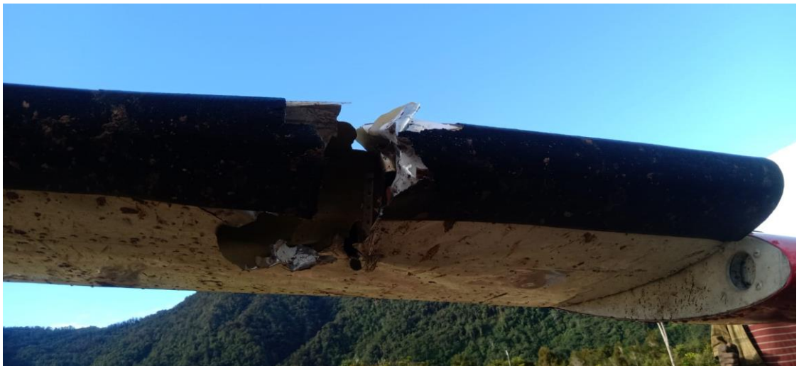
Figure 6: Damaged leading edge of left horizontal stabilizers
