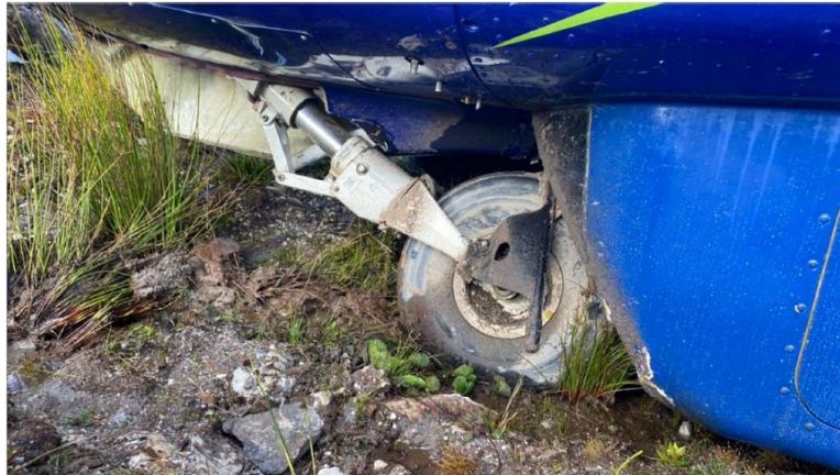
Figure 3: Damage to the forward cargo door
