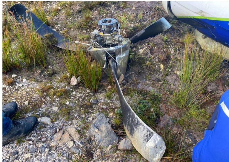
Figure 2: Damage to the propeller
