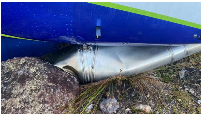
Figure 5: Damage to the engine exhaust
