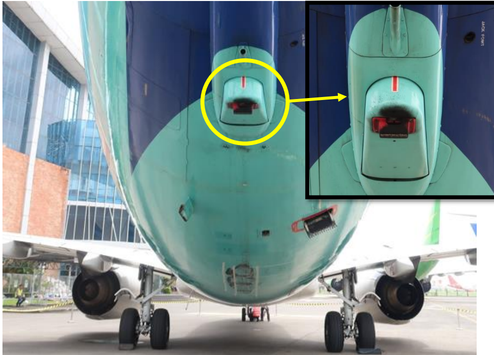
Figure 3. Deflected tailskid damper
