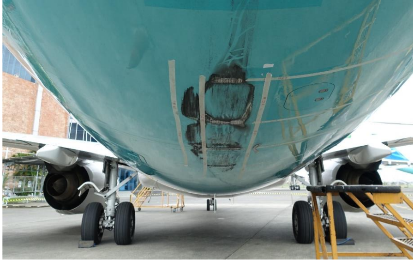
Figure 1. Scratches on lower surface of the aft fuselage skin (view looking forward)
