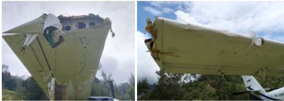
Figure 1 Damage on the left wingtip and leading edge
