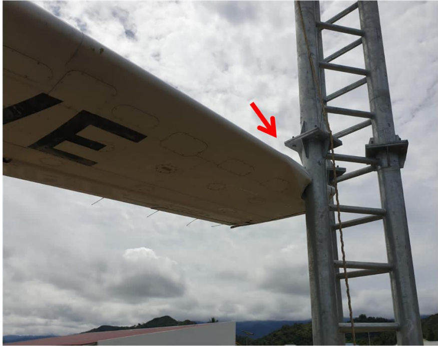
Figure 3: The left-wing leading edge impacted floodlighting pole
