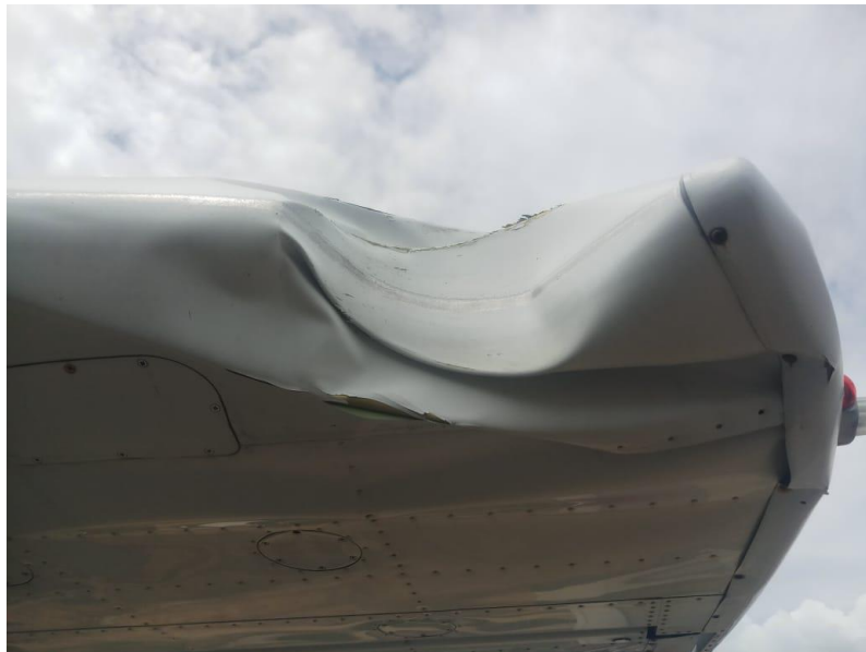
Figure 4: The damaged of the left-wing leading edge
