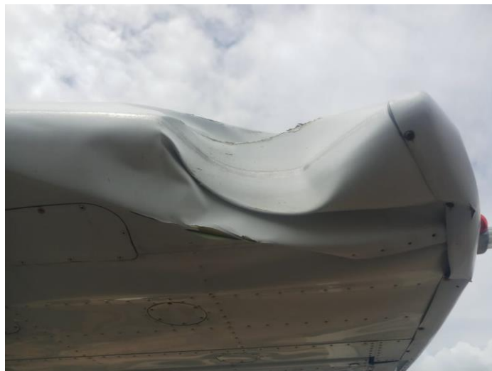
Figure 4: The damaged of the left-wing leading edge
