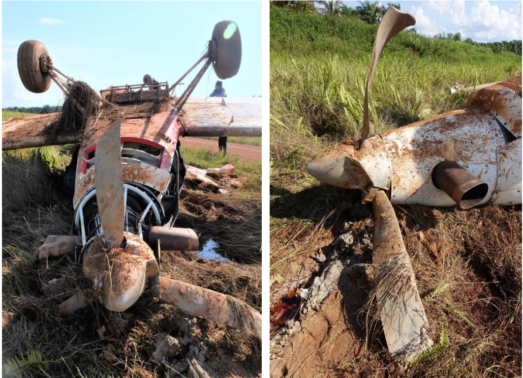
Figure 2: Damage to the aircraft nose and propellers
