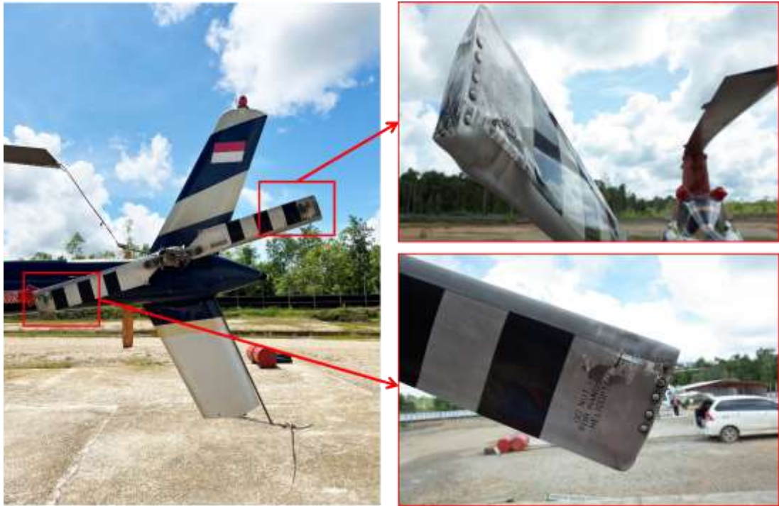
Figure 4: The tail rotor blades damaged
