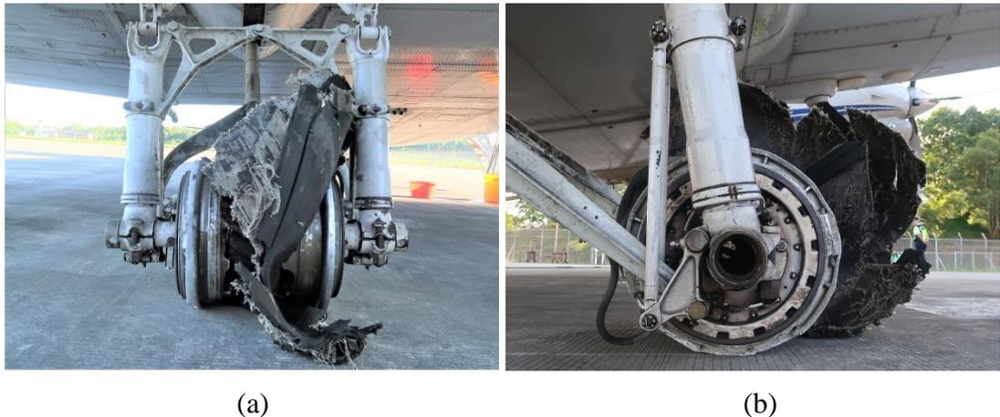
**Figure 1: Damage to aircraft right landing gear**
