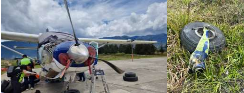
Figure 1.1 Damage to the Aircraft propeller and nose wheel strut detached
