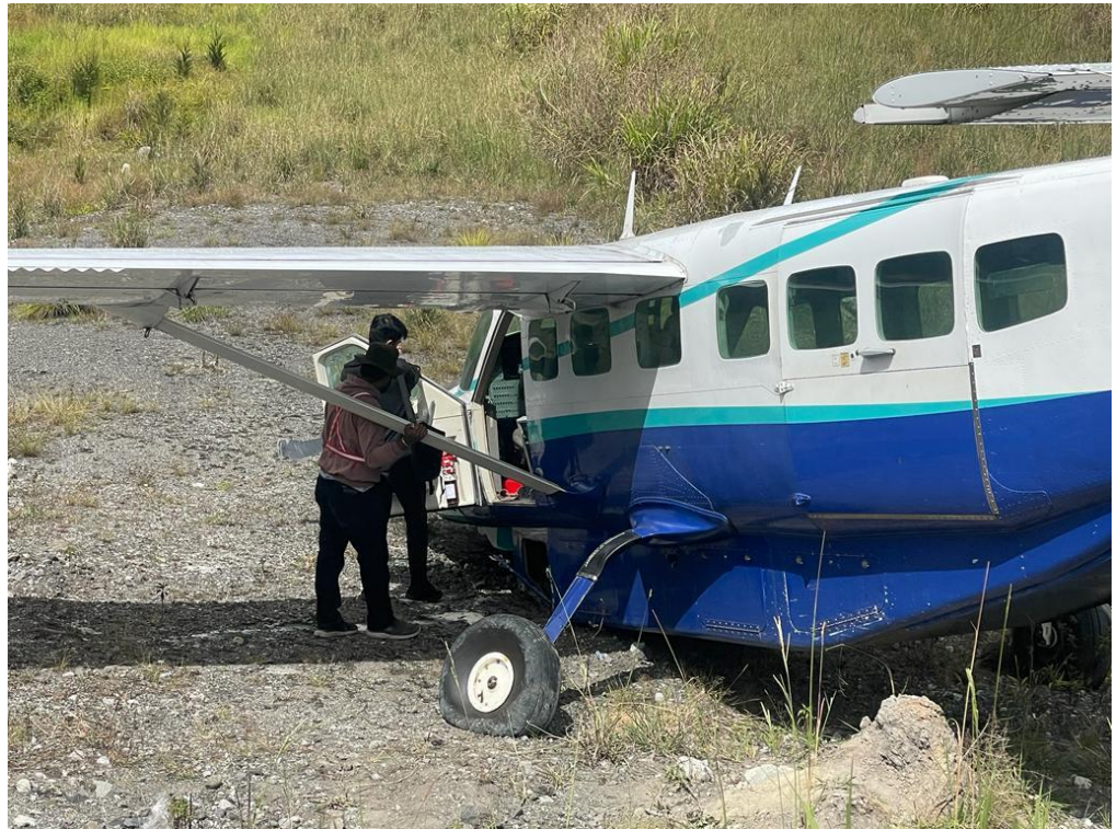
Figure 2: Damage to the left main landing gear
