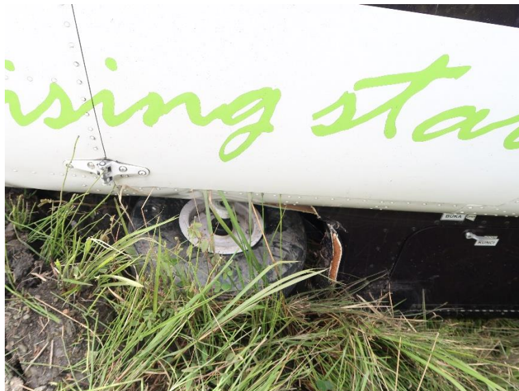
Figure 5 The damaged of the nose landing gear
