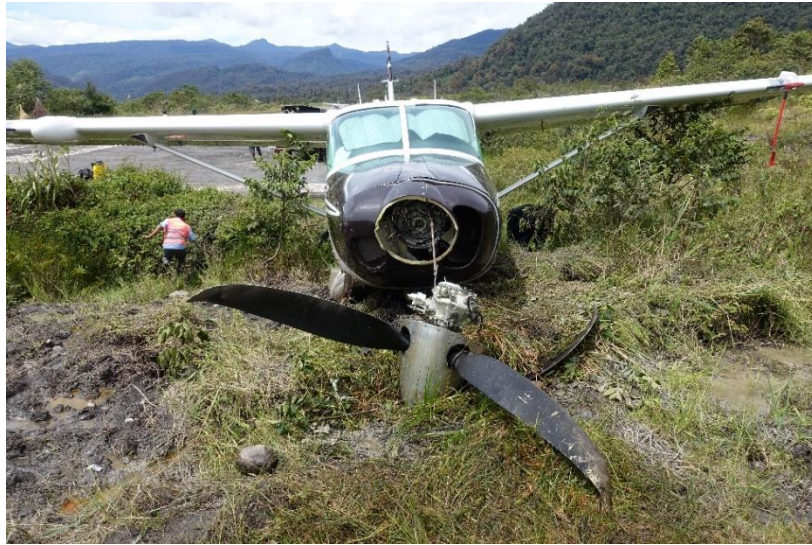
Figure 4 The damaged of the propeller and the blades
