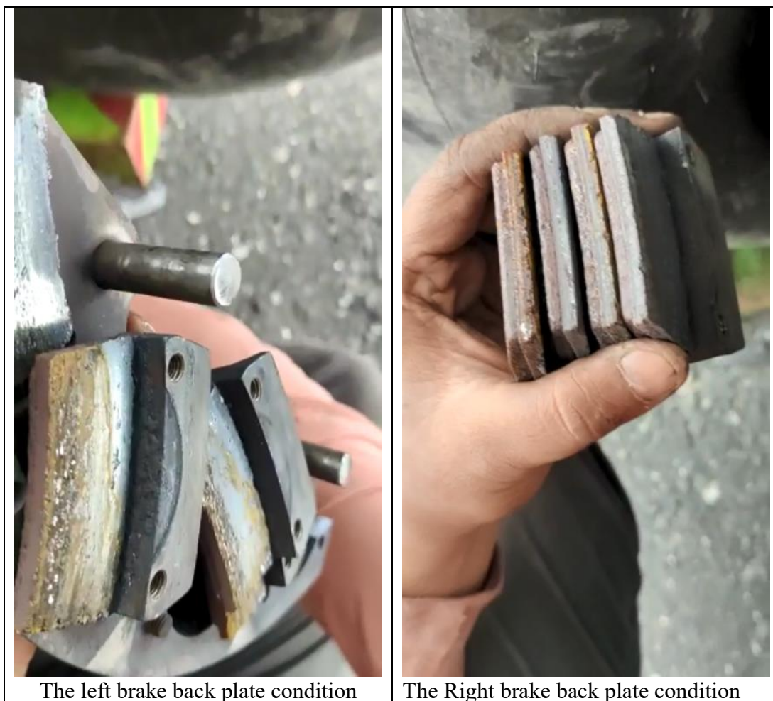
Figure 10: All brake linings condition
