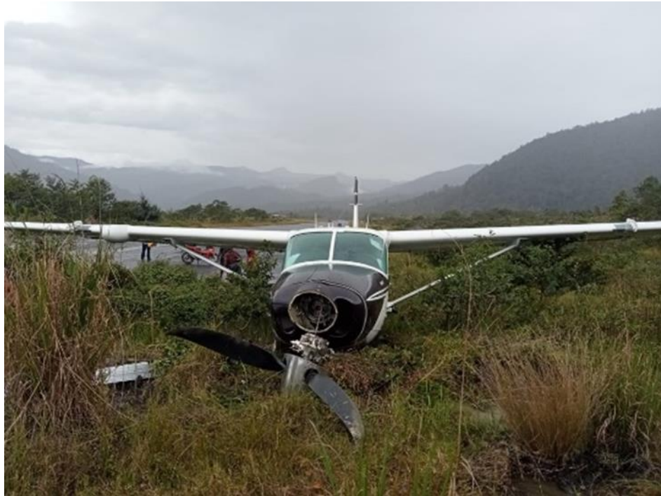
Figure 2: The damaged of the nose section and the propeller
