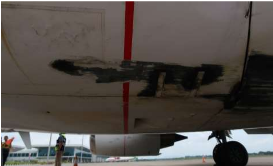
Figure 1 Scratches on lower surface of the left engine cowling
