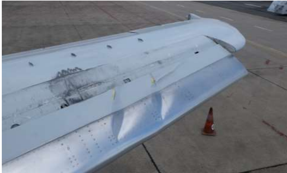
Figure 4 Wrinkles and dents on the wing upper surface
