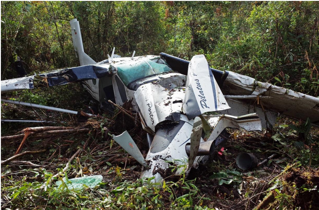
Figure 9: The damaged nose section of the aircraft
