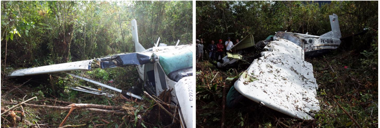
Figure 10: The damaged wings
