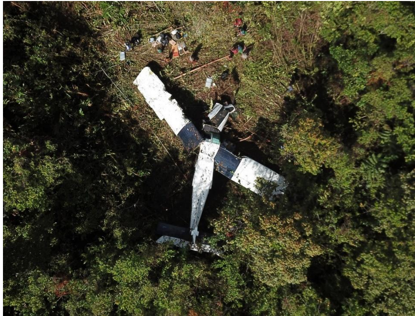
Figure 8: The wreckage condition from above
