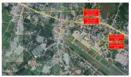
Figure 2: The estimated debris location of the right engine of PK-JRW
