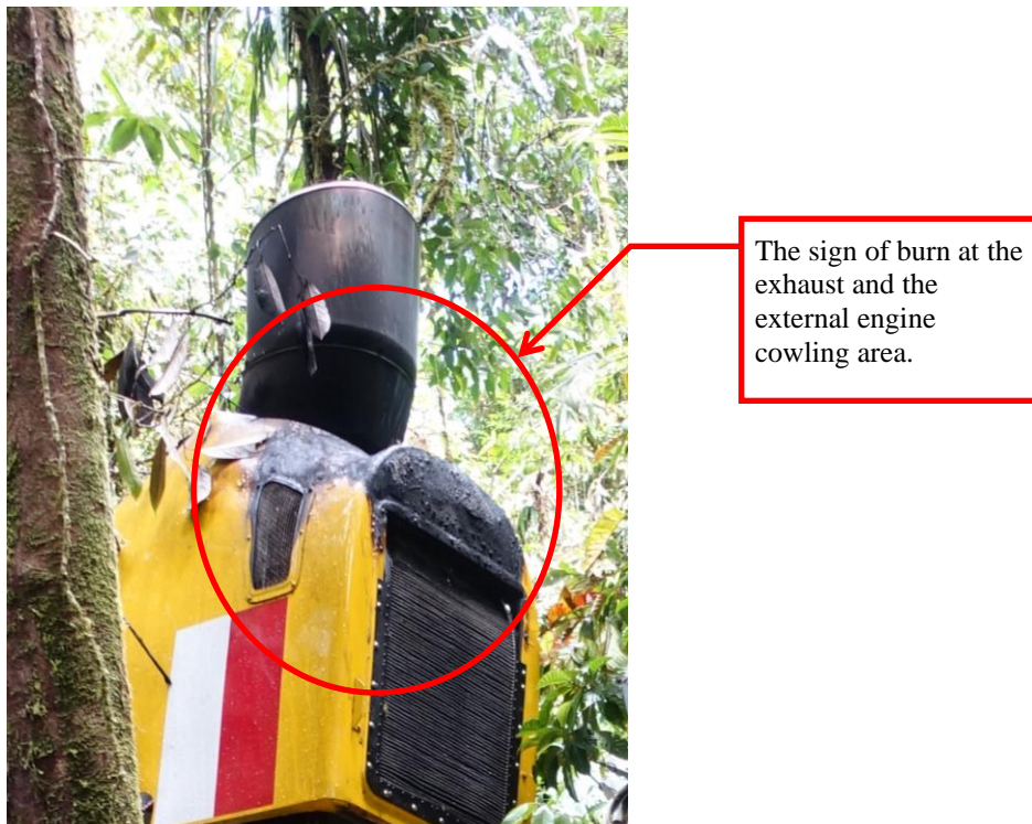
Figure 5: The sign of burn on the near engine area
