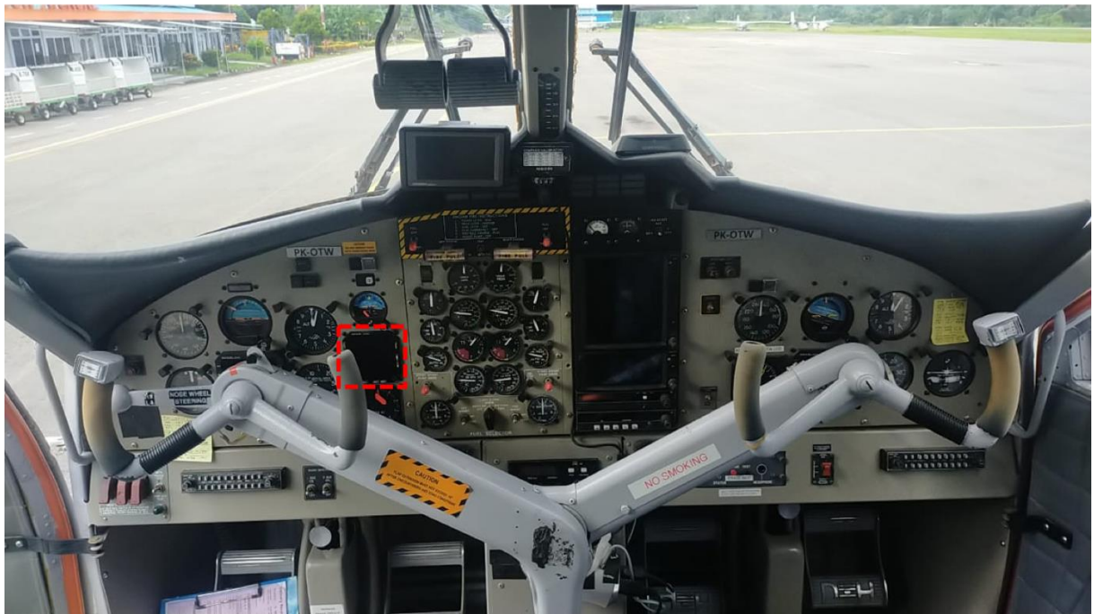
Figure 2: The ST3400 TAWS/RMI location (red square)
