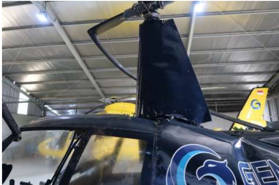
Figure 3. Main rotor mast cowling bent forward
