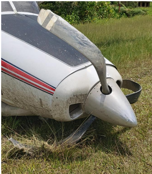
Figure 6: The damaged of the propeller blades
