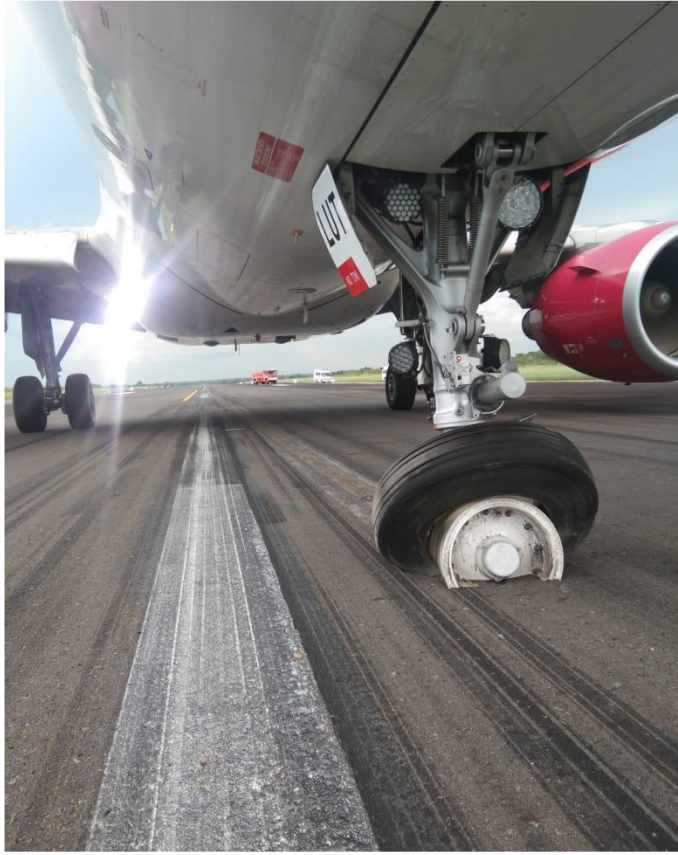
Figure 1. Nose landing gear damage
