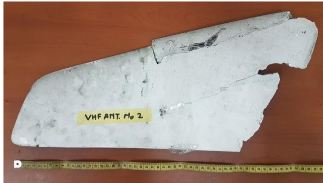
Figure 2: The broken VHF antenna number 2
