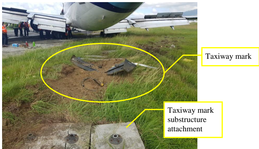
Figure 20: The damage of the taxiway sign board
