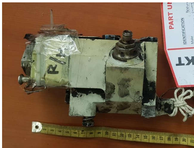
Figure 13: The right manifold of shimmy damper assembly
