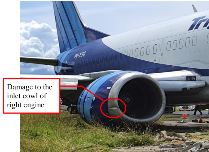
Figure 4: Dent on the right engine inlet cowl
