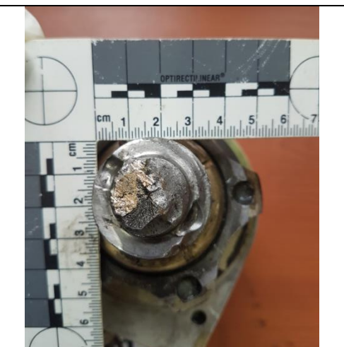
Figure 10: Broken piston of left shimmy damper
