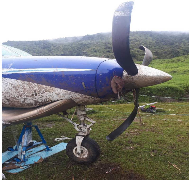
Figure 5: The damaged of the propeller blades
