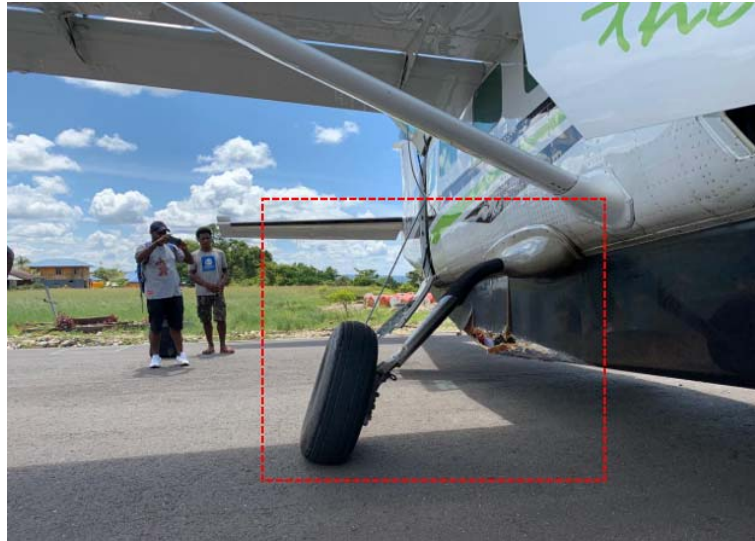
Figure 1: The bent of the right main landing gear strut
