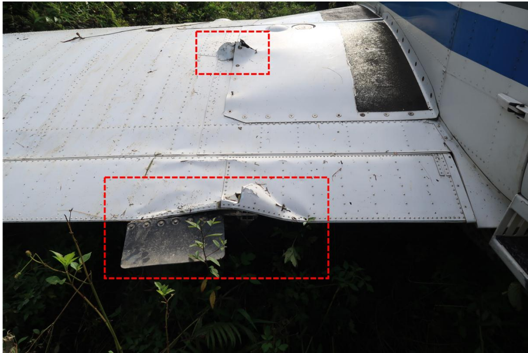
Figure 10: The damaged of left wing
