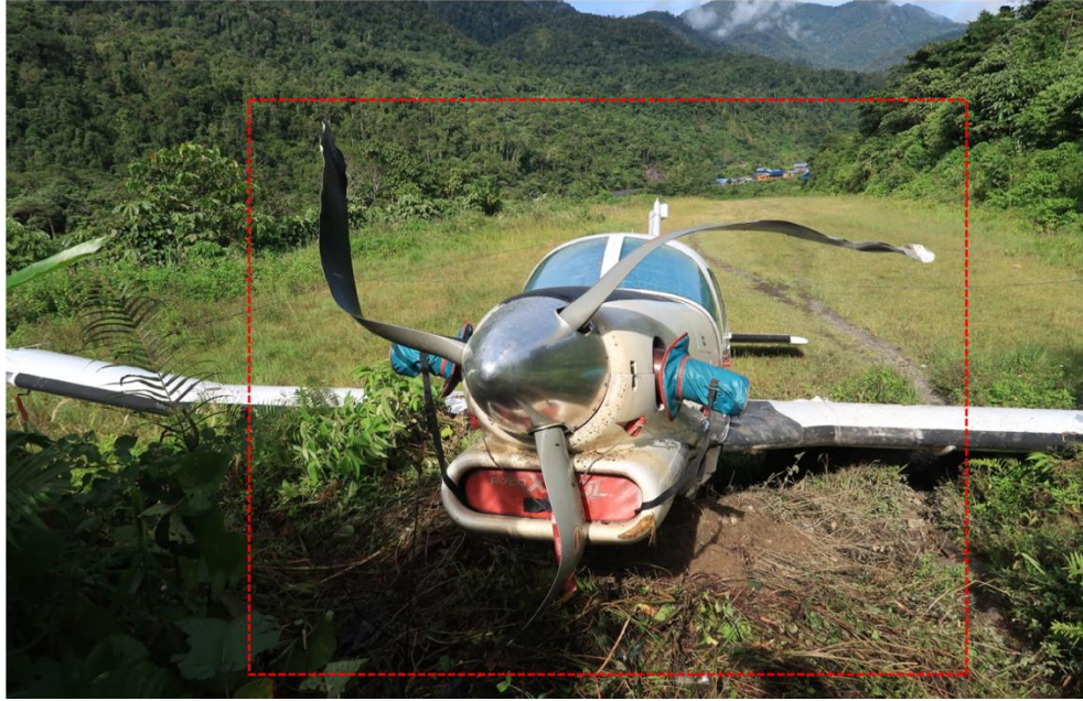
Figure 8: The damaged propeller blades
