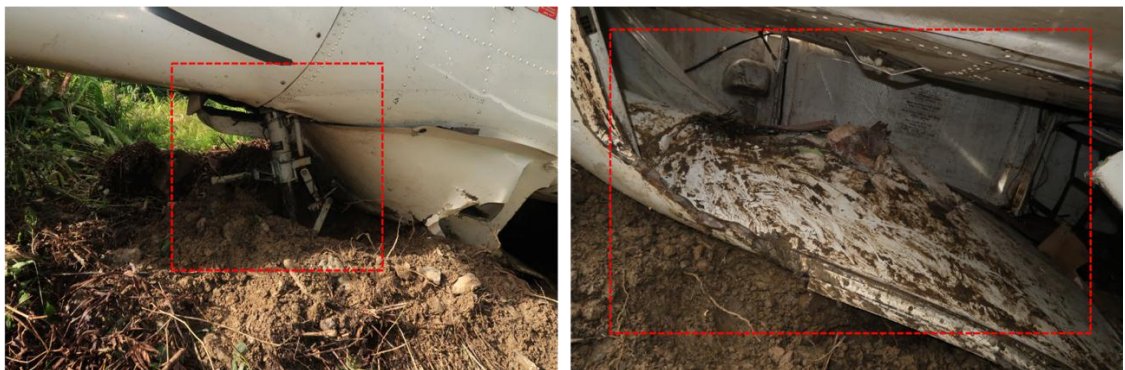
Figure 9: The bent of nose landing gear strut (left picture) and the damaged of cargo pod (right picture)
