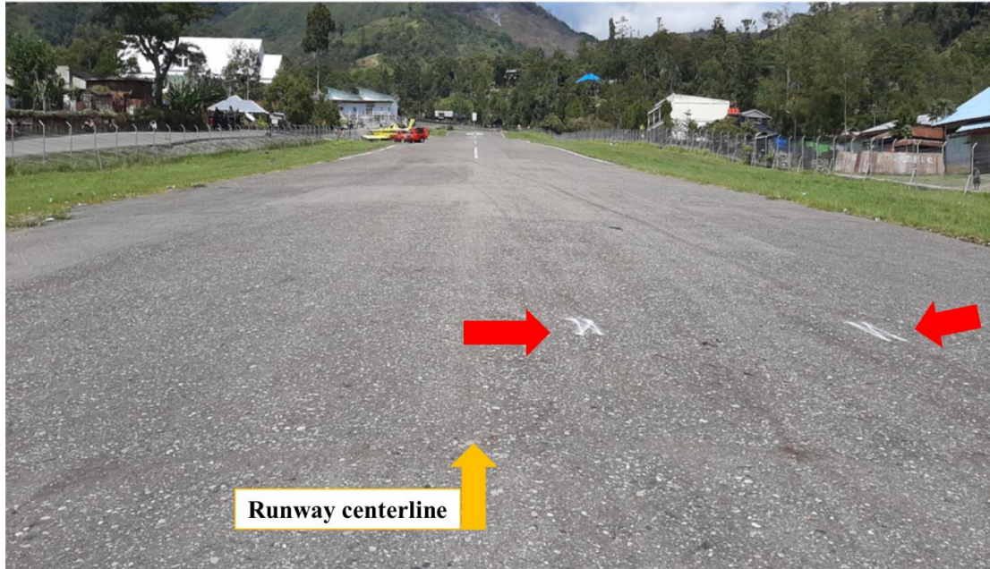
Figure 4: The beginning of braking marks on the runway (red arrows)
