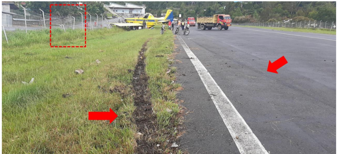
Figure 5: The wheel marks (red arrows) and the first damaged fence (red dotted square)
