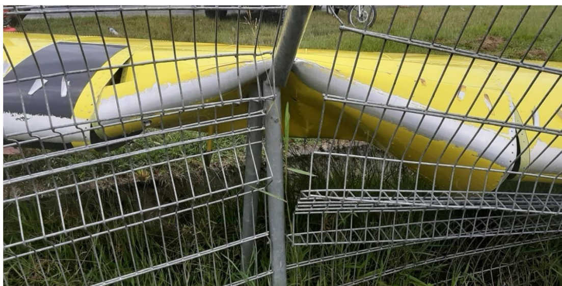
Figure 9: The damaged left-wing leading edge
