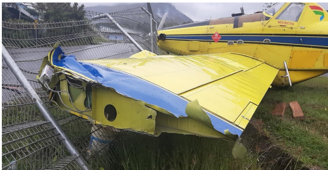
Figure 8: The damaged left-wing tip
