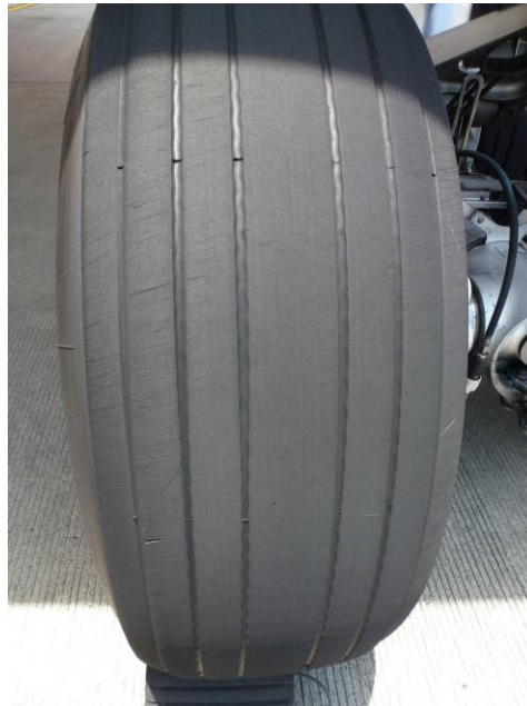
Figure 2: Striation mark in lateral direction on tire surface.
