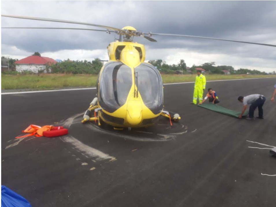
Figure 5: The helicopter position and the scratch marks
