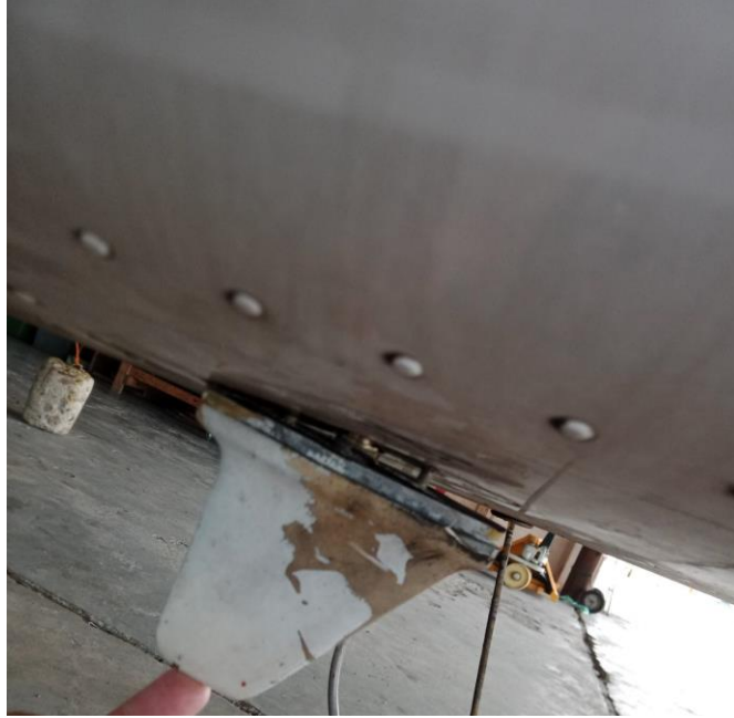
Figure 4: Damage on transponder antenna
