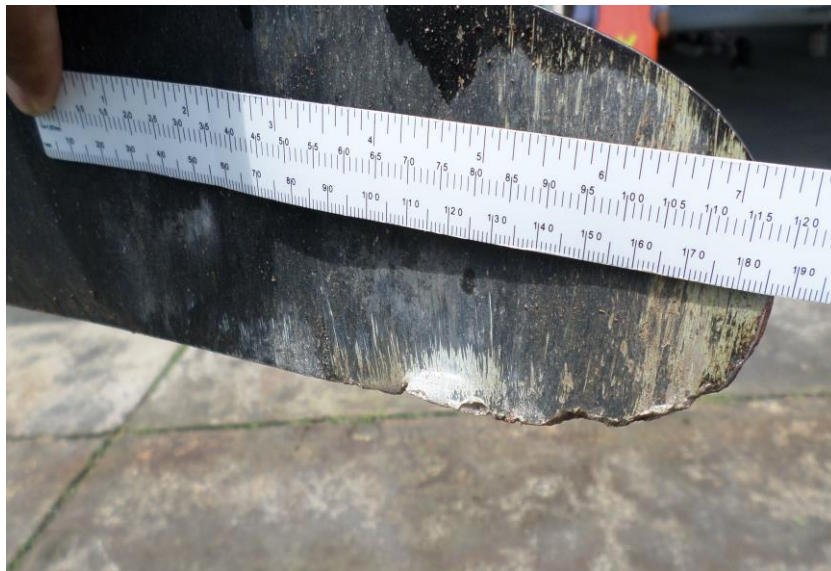
Figure 3: Damage on propeller blade
