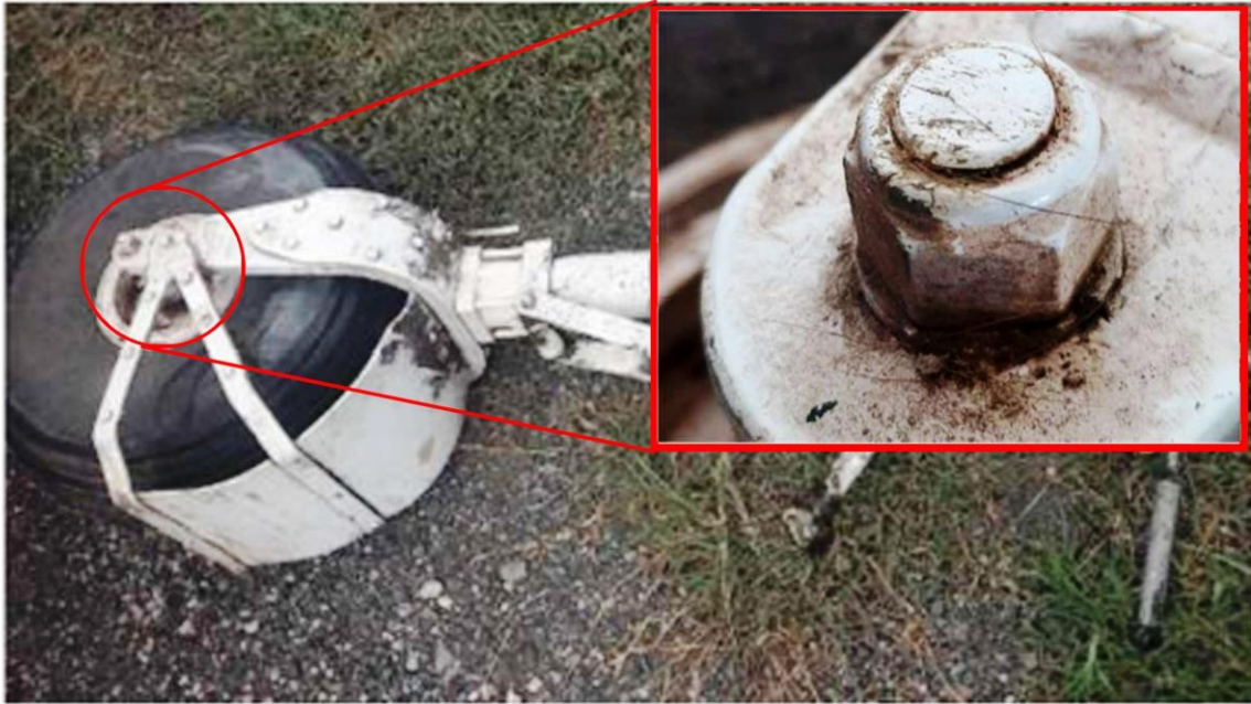
Figure 7: Boar's Furs found in the Nose Wheel Fork
