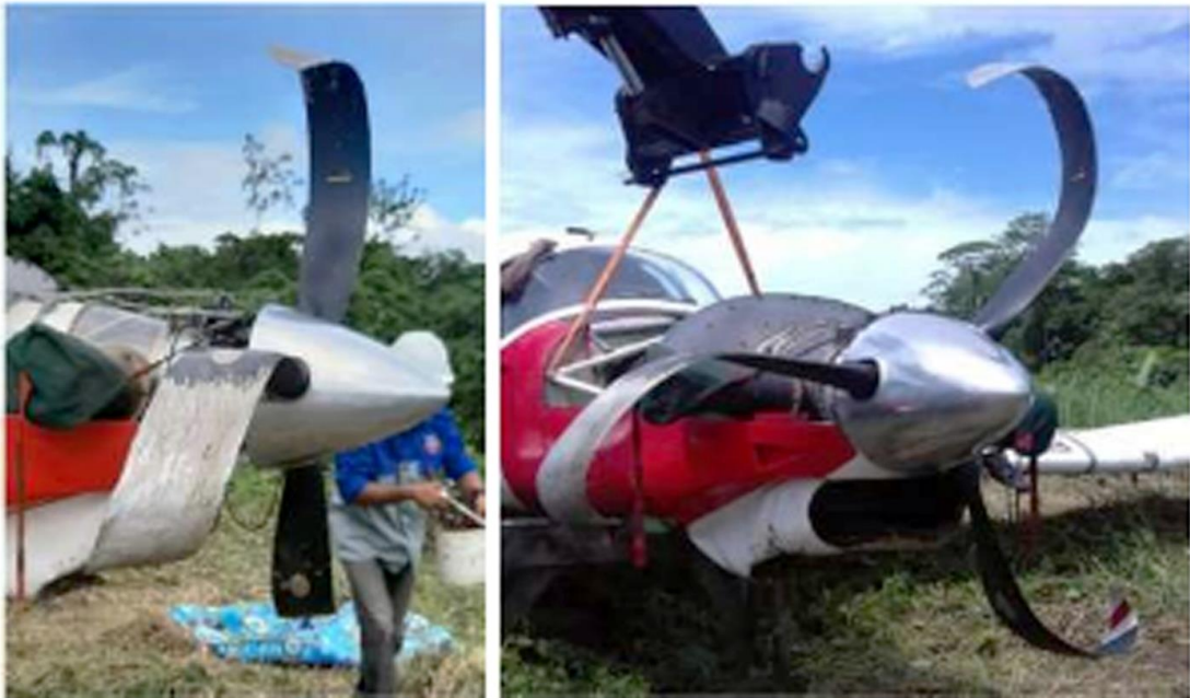
Figure 2: Damage to the propeller blades
