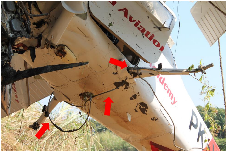
Figure 5: The power line cable caught in the main landing gear struts (red arrows)
