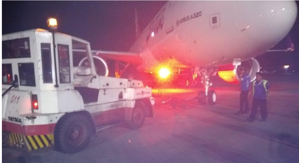
Figure 3: The position of the towing tractor and the aircraft after the accident
