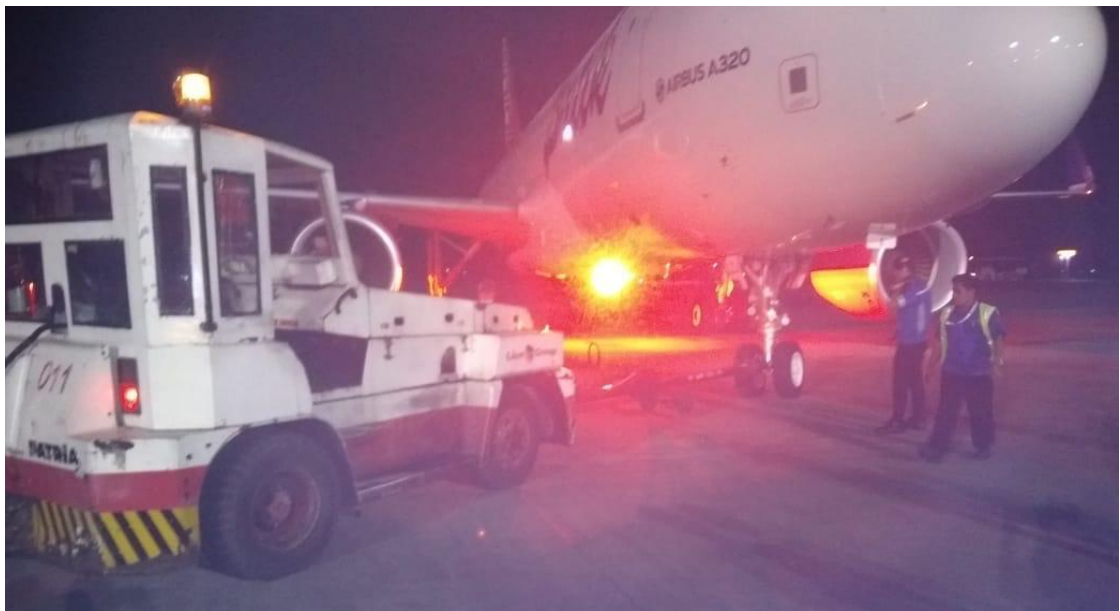
Figure 9: The position of the towing tractor and when the aircraft stopped after the accident
