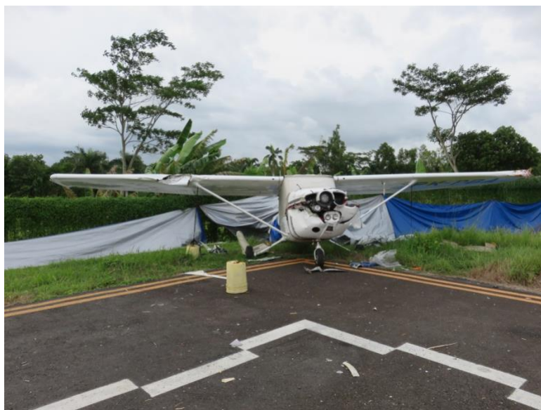
Figure 5: The one aircraft that was parked on the corner of the apron damage The two aircraft damage inside the hangar is shown in the figure below.
