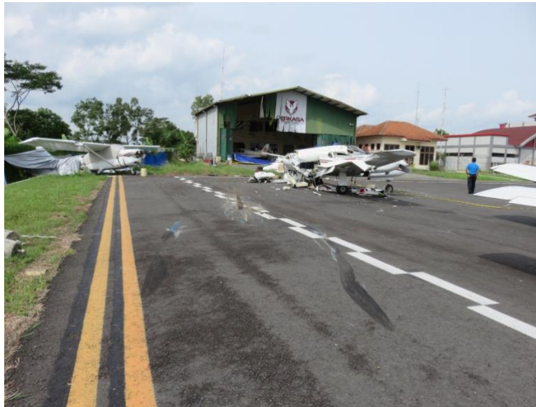
Figure 8: The landing gear and propeller marks toward the hangar
