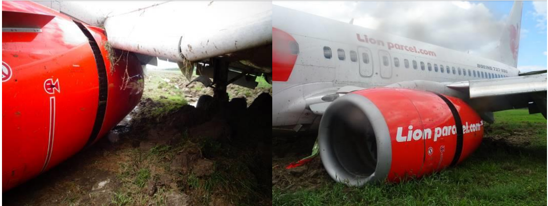
Figure 9: Left and right engine thrust reversers condition
