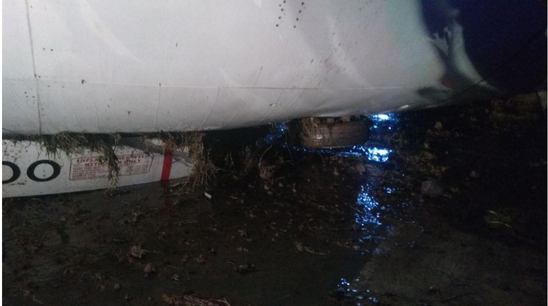
Figure 1: The nose landing gear collapsed backward
