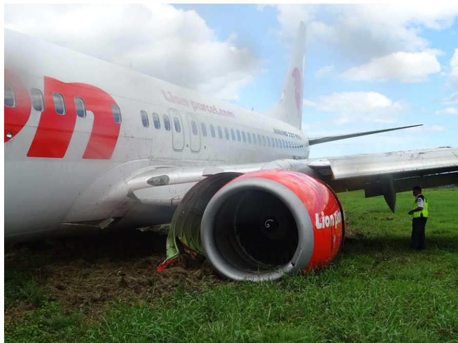
Figure 2: Damage on the right engine cowling
